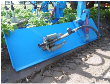
DABb injectors deliver with minimum soil disturbance
