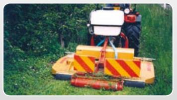
The **herbicide spraying system XID** may be mounted to many SEPPI mowers. High-precision nozzles come with adjustable spraying direction.
