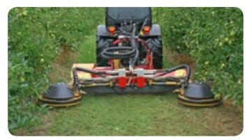
The **outrigger XSC** is specialized for inter-row mowing. The double XSC outrigger also adapts to row widths. This makes mowing much faster and more efficient.
