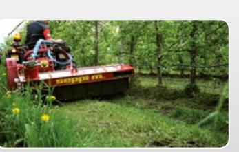
The **conveyer belt XTR** deposits grass to the right of the mulcher. This inhibits the growth of the grass and allows to reduce the use of chemicals.
