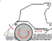
Adjustable anvil bar & crushing grid to adjust the degree of mulching
