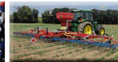
Harrow, 9m working width with pneum. Seeder
