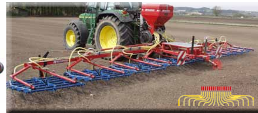
Harrow, 12m working width with pneum. seeding machine „Air 16“
