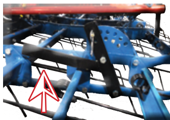
10 hole adjustment of tine aggressiveness
