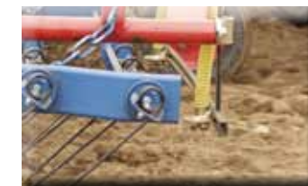
Harrow, 5 m working width, introduction of cover crop with baffles on harrow field mounted
