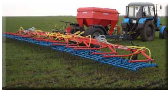
12m Harrow with seeding machine Air Cart Trailer 3000 liter volume
