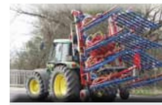
Harrow, 9m working width, transport position (shear folding)
