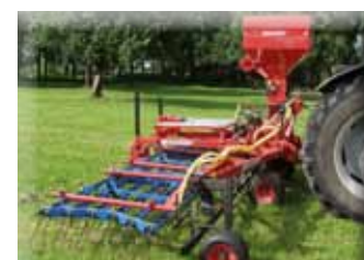
Harrow with 6m working width in connection with the seeding machine „Air 8“ for overseeding the grassland
